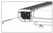
4. If the striding belt has moved to the left, turn the left tension bolt 1/4 turn clockwise and then turn the right tension bolt 1/4 turn counter-clockwise to tart striding belt tracking back to center of roller. Repeat adjustments until the striding belt appears centered. Allow the machine to continue running for several minutes to observe if tracking remains stabilized.
